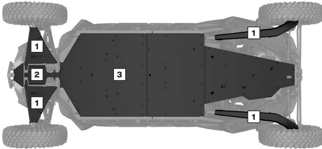
Our plastic plates glide smoothly and silently over obstacles, offering great protection in rough terrain. Made of abrasion-resistant thermoformed  $\frac{3}{8}$ " (10 mm) thick High Molecular Weight Polyethylene (HMWPE).
